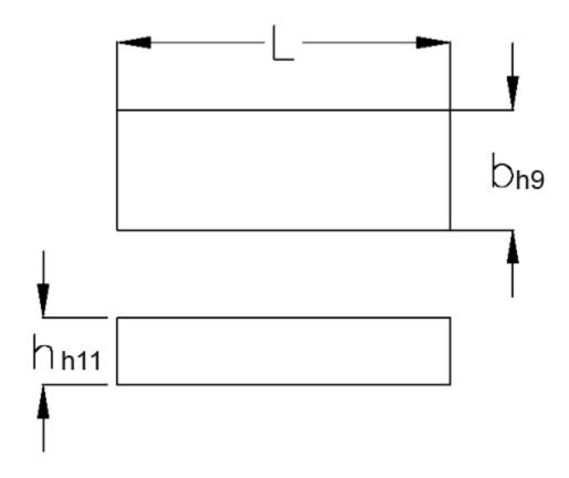
b = 20 h = 12 L = 70 Tolerance b = 0.052 Tolerance h = 0.110 Tolerance L = -0.3
